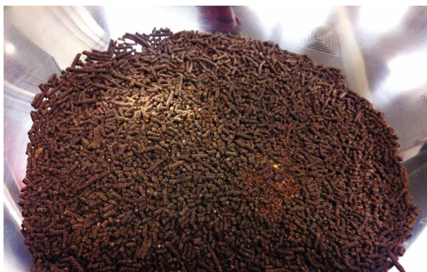
Fishmeal made from nutrients removed from wastewater treatment
